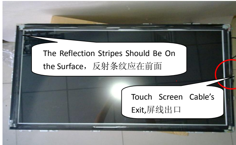
(The front view after sticking the touch screen, 贴上触摸屏后的正面视图)
