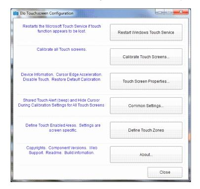
The following is a description of each of the buttons located in the Elo Touch Screen Configuration application:
