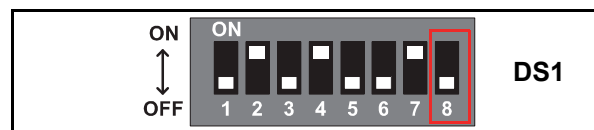
Figure 2-4 ICB DIP Switch Setting 2
