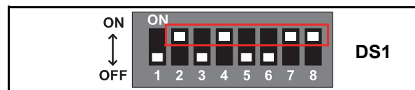
Figure 2-3 ICB DIP Switch Setting 1
