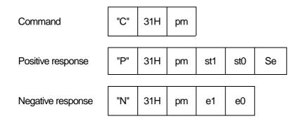
Negative response is sent against Status request command if mechanical failure remains from the prior operation.
