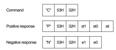
When this command is received, ICRW reports the condition of an I2C memory card by byte of "stj". While a power supply is supplied to the card, the ICRW monitors VCC (the power supply line of the card). An error "60" is returned when a power failure is detected.
