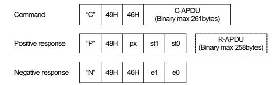
In the protocol T=1, this command is used when the last data are transmitted.
