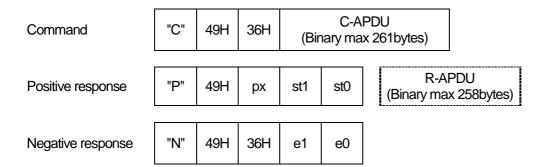
In the protocol T=1, this command is used when the last data are transmitted.
