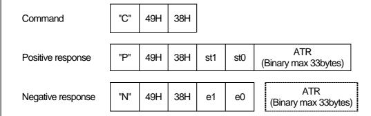
ICRW sends a reset pulse, keeping the status of the IC contact activated (VCC,CLK), then returns response upon receiving "ATR" again. The reset pulse width is around 12msec. This command gives effect to change into the specific mode.
