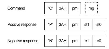
Control command to accept/inhibit card entry. ICRW sends response upon receipt of this command. ICRW status should be recognized by Status request command from HOST.
