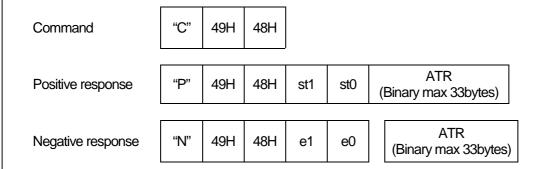
ICRW sends a reset pulse, keeping the status of the SAM activated (VCC,CLK), then returns response upon receiving "ATR" again. The reset pulse width is around 12msec. This command gives effect to change into the specific mode.
