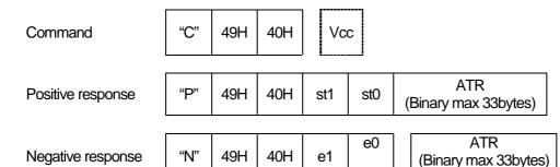
To activate SAM, power (VCC) and clock (CLK) are supplied and reset (RST) is released.
