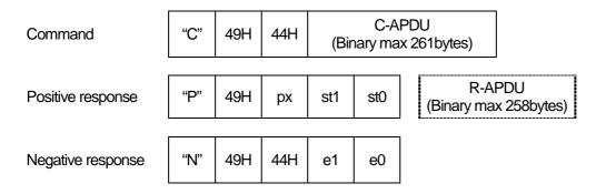
This exchanges data between SAM by protocol T=1. ICRW sets C-APDU to Information field and transmits to SAM.
