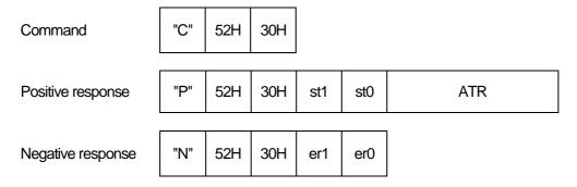
This command activates the memory card. ICRW supply power (Vcc) and clock(CLK), and assert reset (RST) signal. Then, the memory card is activated and return ATR. ICRW returns a negative response when proper ATR isn't received from the memory card. An error code "60" is returned when a power failure is recognized while a power supply is supplied to the card.
