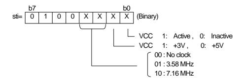
While SAM is being activated, ICRW is monitoring VCC to detect excess current of VCC. If excess current should be detected before receiving this command or during execution of this command, error code "60" is sent.
