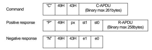
This exchanges data between SAM by protocol T=0. About the format of C-APDU, see ANNEX 4. ICRW sets C-APDU to chipdata and transmits to SAM.
