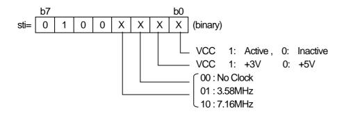
While ICC is being activated, ICRW is monitoring VCC to detect excess current of VCC. If excess current should be detected before receiving this command or during execution of this command, error code "60" is sent.
