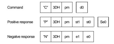
This is to check ICRW in maintenance. Operation checks can be done by this command for the motor, the solenoids, the switch, and the sensors.
