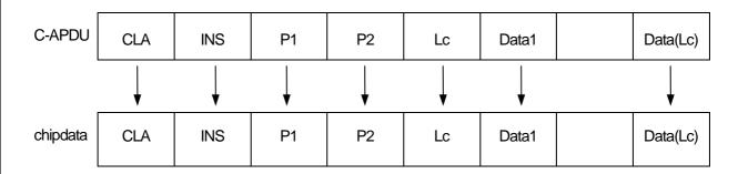
ICRW sets to R-APDU chipdata which received from ICC, and transmits to HOST.
