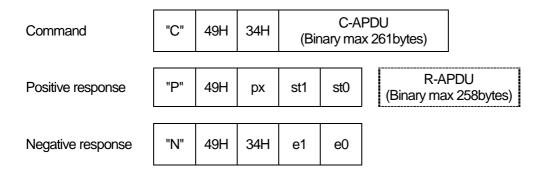
This exchanges data between ICC by protocol T=1. ICRW sets C-APDU to Information field and transmits to ICC.
